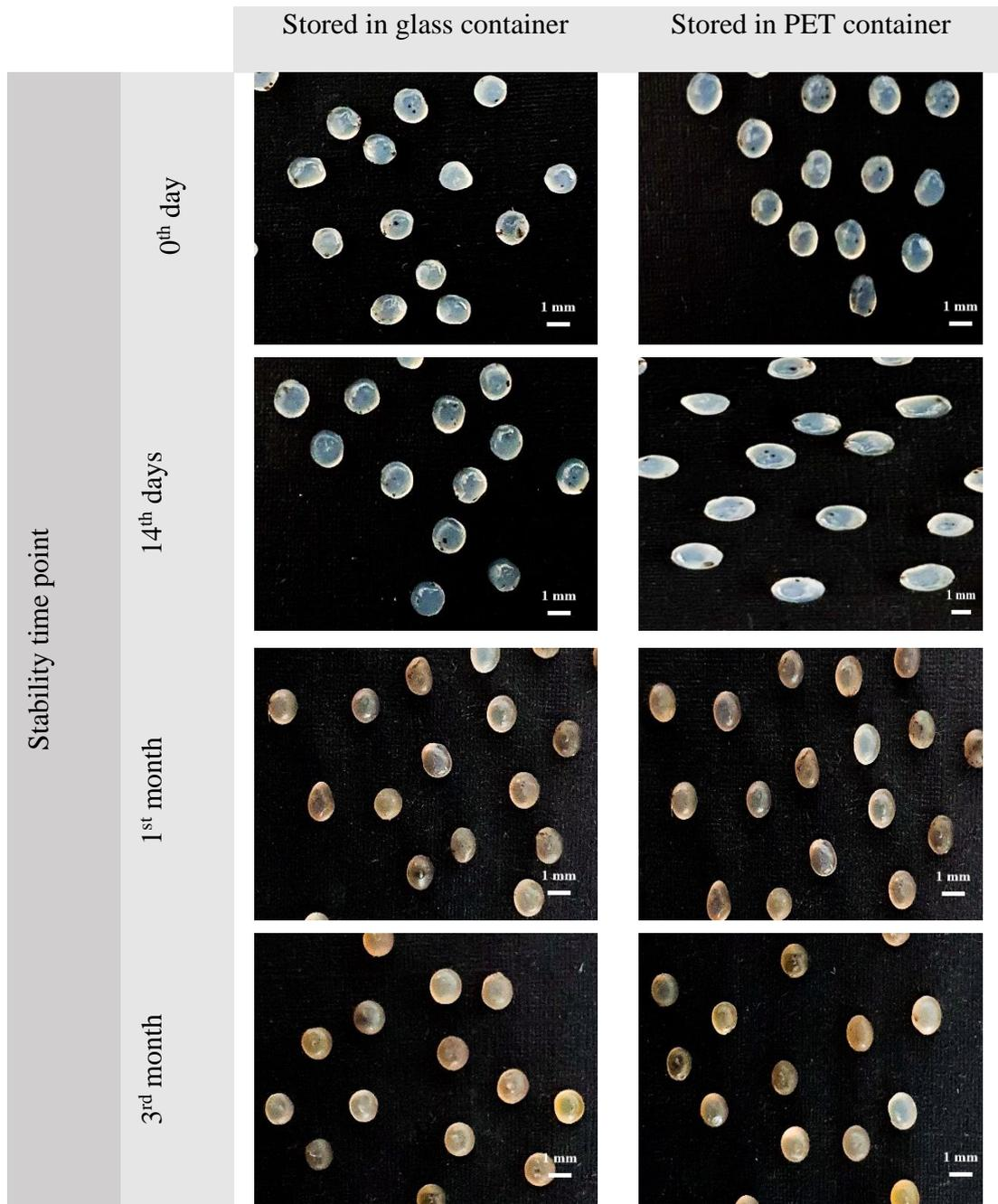
Figure 4. The physical appearance of RJ beads stored in accelerated stability chamber at four stability time points (0-day, 14-day, 1-month and 3-month)
