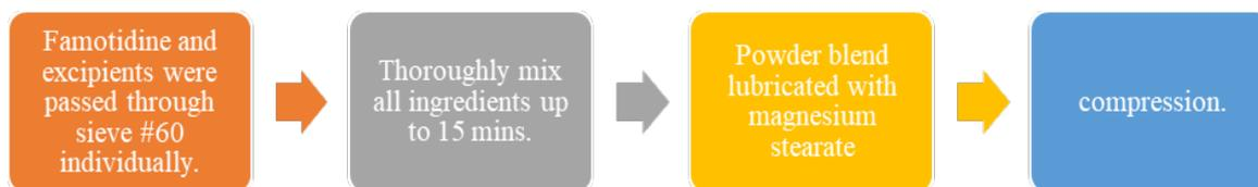
Figure 1: Preparation of core tablet.
