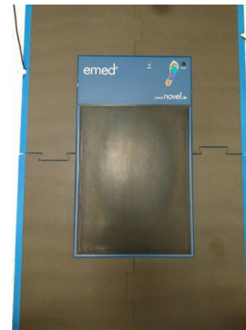
Figure 2: The sensor area at the middle of the platform
