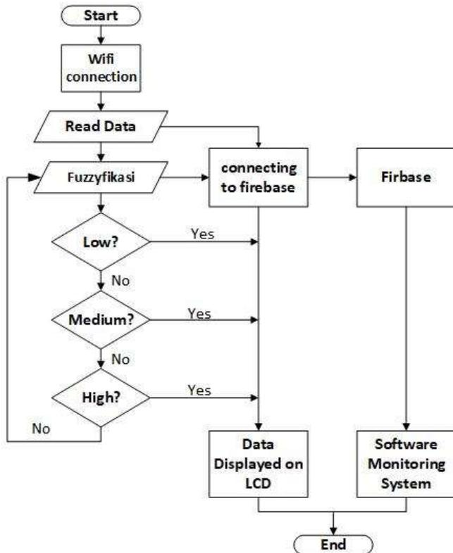
Fig. 2 Flow chart of the system work process
