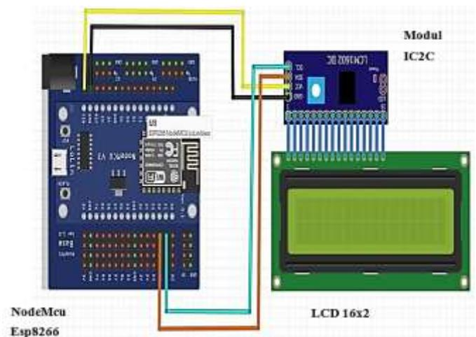
Fig. 3 Circuit Schematic Displaying Data
