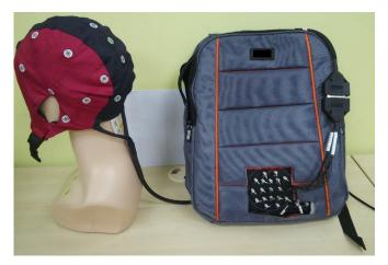
Figure 2. EXG Brain Marker Mobile EEG Device in Bag pack.
