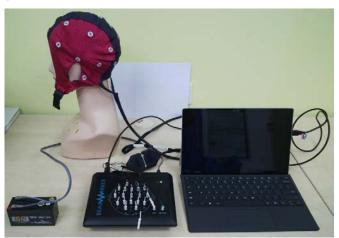
Figure 1. EXG Brain Marker Mobile EEG Device
