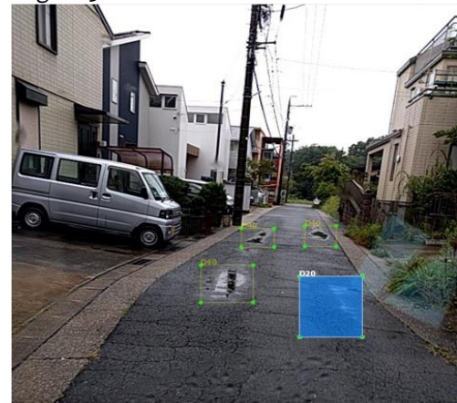
Fig. 3 Bounding box are drawn to label the objects
