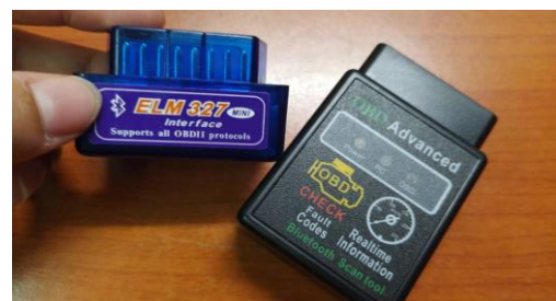
Fig. 1: ELM 327 with Bluetooth interface
