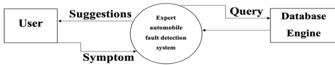
Fig. 1 Dataflow Diagram of the Expert automobile fault detection System
