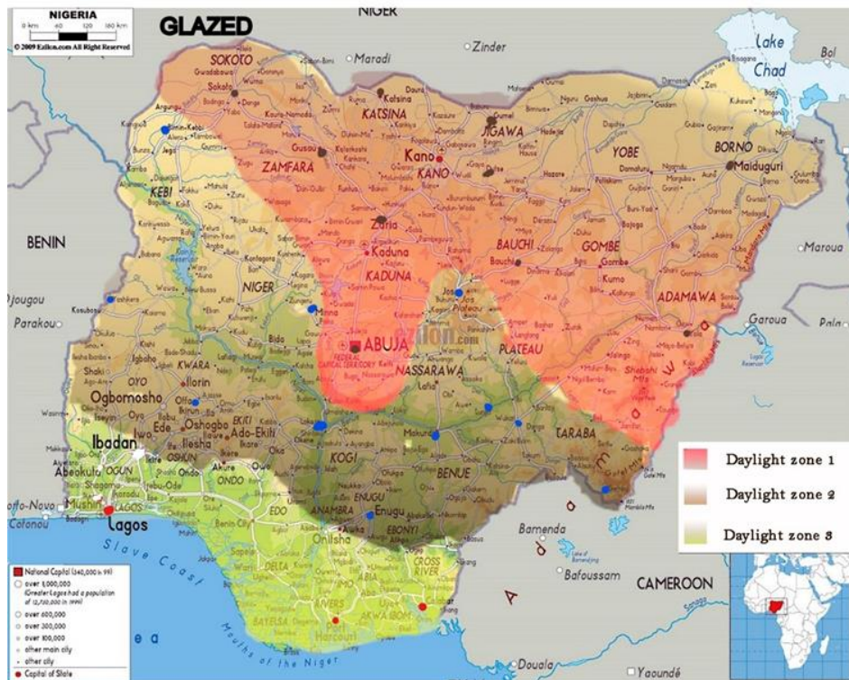
Fig. 4: Map of Nigeria showing the Three Daylighting Zones for Glazed classrooms according to the 3 Cluster classification schemes (Source: Salisu, 2015).
