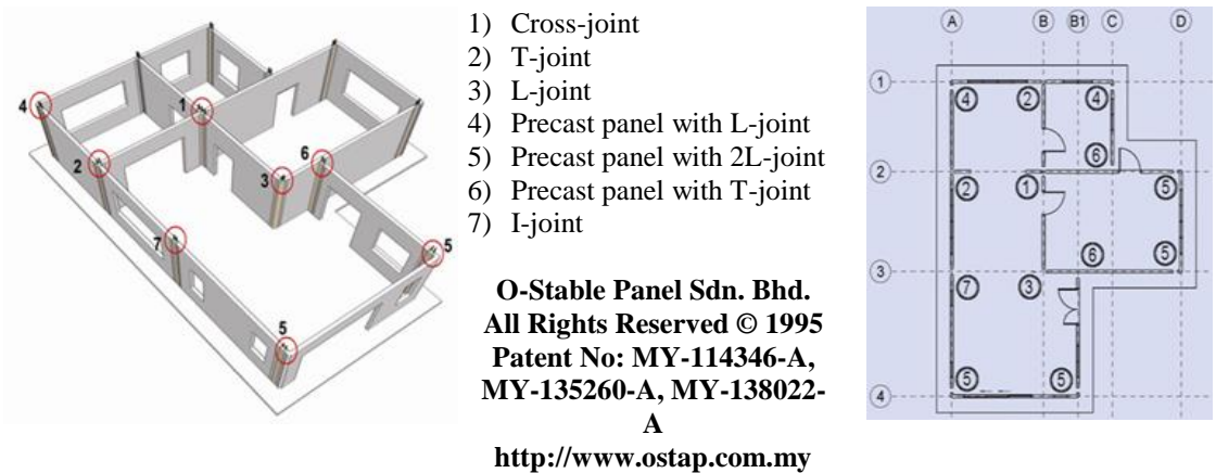
Figure 4 Plan of Standard Detail of Wet Vertical Joints ( Baktian Sdn. Bhd., 2011 )
