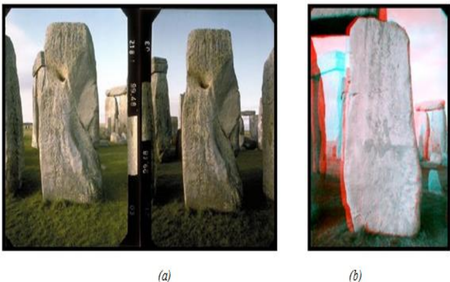
Figure 2: The stereo-photography of Stonehenge taken with Wild P31 metric camera equipped with 100mm focal length lens. (a) Stereo pairs of images (b) The overlapping of a pair of image. (Courtesy: Paul Bryan, the Metric Survey Team, English Heritage)
