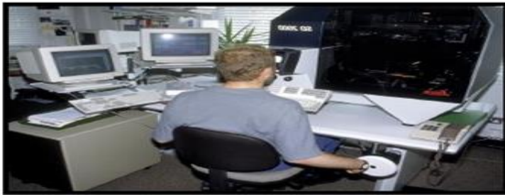
Figure 5: The plotting process using analytical plotter Leica SD 2000.
