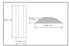
Fig.1: Schematic of Typical Circular Road Hump (Source: Johnson and Nedzesky, 2004)
