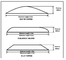
Fig.3: Typical Design of Road Hump (Source: Malaysia Ministry of Work, 2011)
