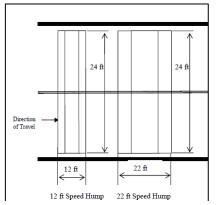
Fig.2: Schematic Drawing of Road Hump (Source: Johnson and Nedzesky, 2004)
