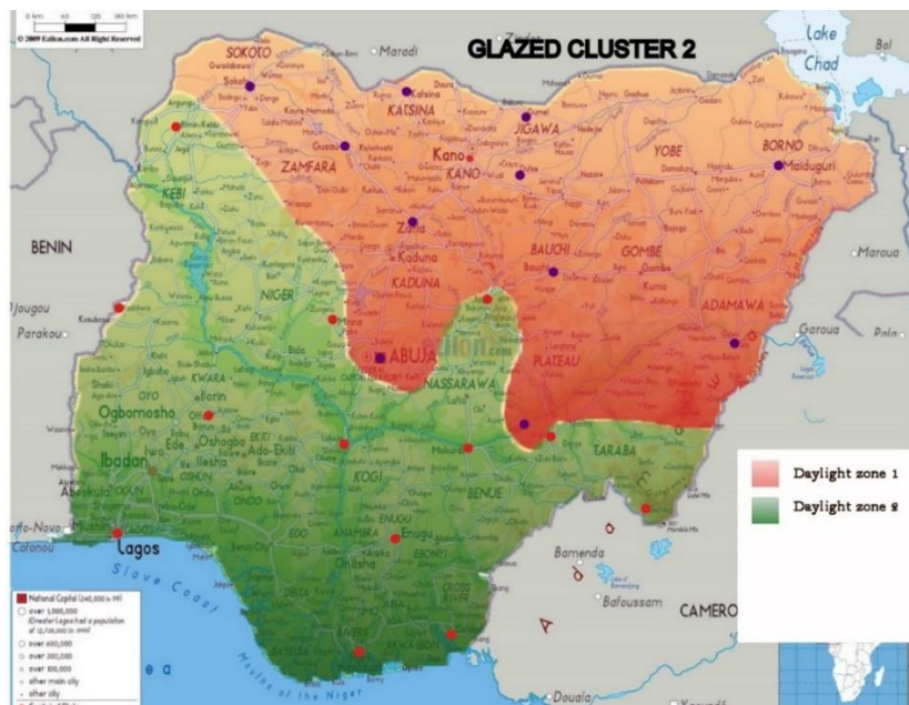
Fig. 8: Proposed Daylighting Zones for Glazed classrooms according to 2 Cluster Hierarchical classification schemes. (Source: Salisu, 2015).
