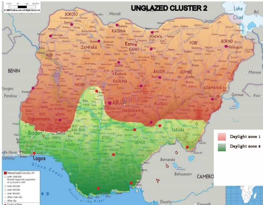
Fig. 9: Proposed Daylighting Zones for Unglazed Classrooms according to 2 Cluster Hierarchical classification schemes.
