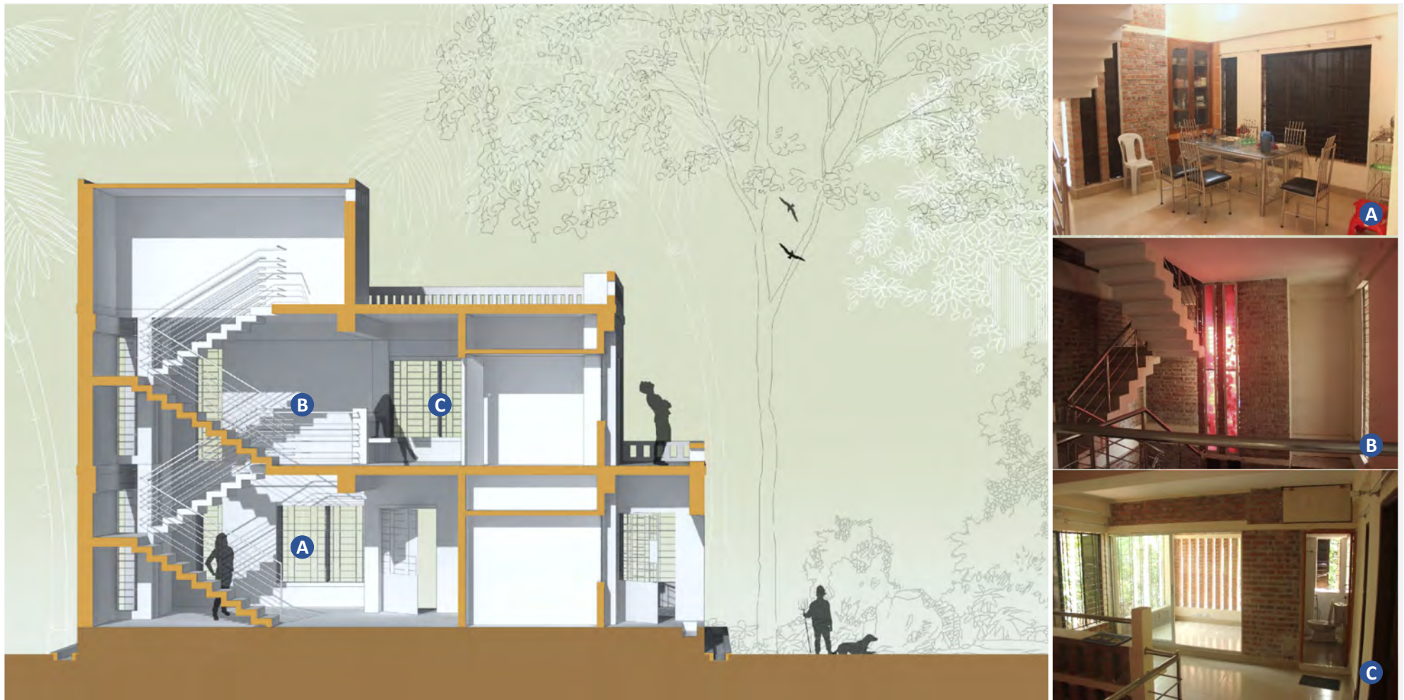
Figure 16: Sectional perspective and photographs showing the double height space connecting the ground floor with the first floor visually for enhanced daylighting, visual connectivity and natural ventilation.
