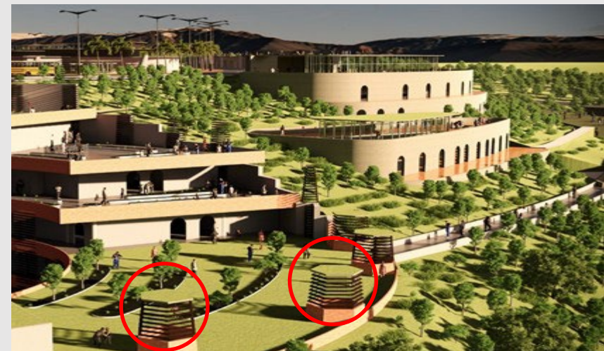
Figure 23: Shafts for the underground non-ventilated spaces (Source: Author)
