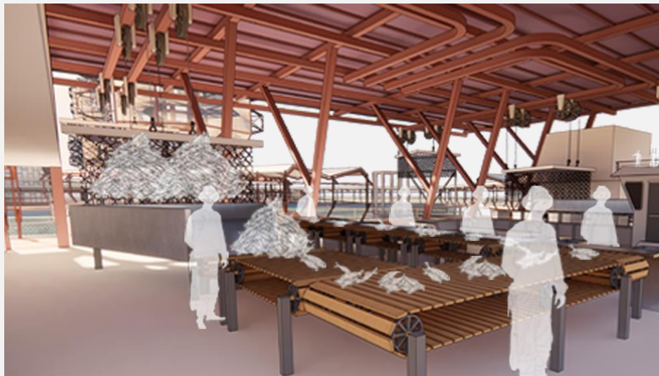
Figure 38: Harvested fish from the cage into the automated conveyor belt for sorting and packaging process
