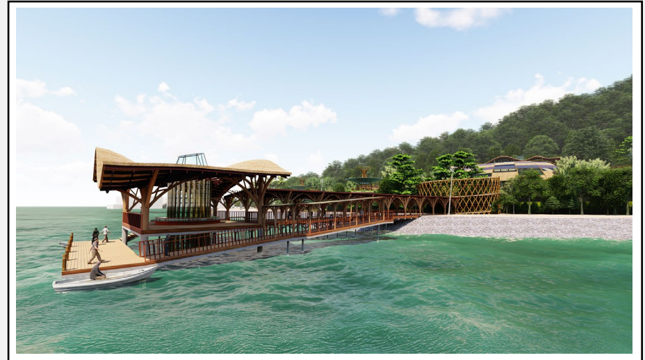
Figure 12: The jetty for tourist is covered with thatch roof and has solar still structure in the middle while the bridge is covered alternately with thatch roof and thin solar film.
