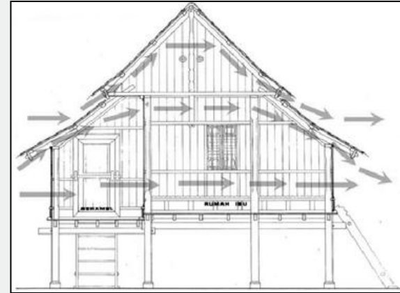
Figure 1: Ventilation Openings in the Roof of Traditional Malay House. (Source: Center of Built in the Malay World (KALAM), 1986.)
