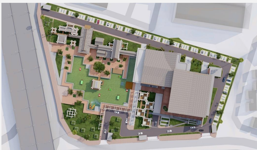
Figure 10: The site plan showing the placement of the urban plaza adjacent to the main road for easy accessibility.
