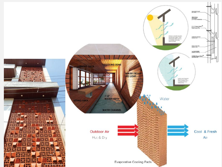
Figure 19: Bricks, shading device and evaporative cooling pads. Source: Author
