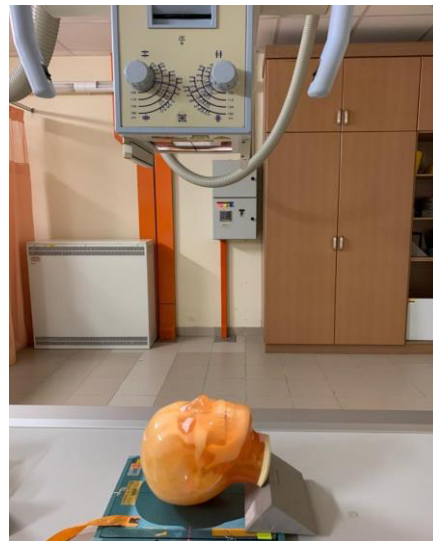
Figure 1. Shows the PBU-50 head phantom on the bucky table with grid (no air gap).
