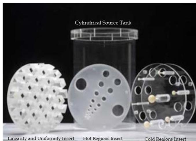
Figure 1 R.A Carlson's SPECT Phantom and inserts (Bailey et al, 2014)
