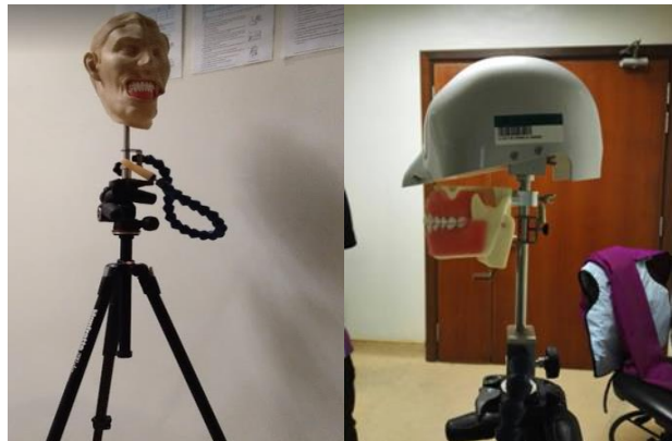
Figure 2. X-Ray Adult Simulator - Manikin Portable Complete with rubber mask (left), without rubber mask (right) and tripod stand
