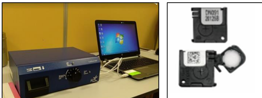
Figure 1. OSLD Microstar Reader (left) and nanoDot OSLD (right)
