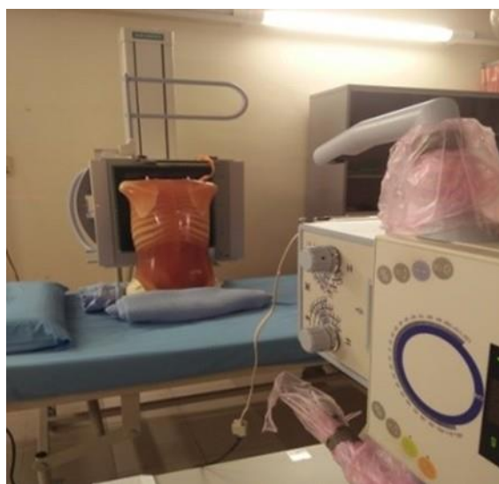
Figure 1. Experimental setup for PA chest radiography
