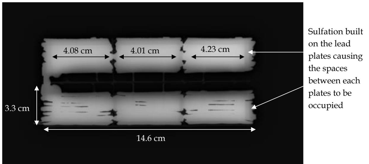
**Figure 2.** Top view of lead acid battery exposed at 125 kVp, 15 mAs
