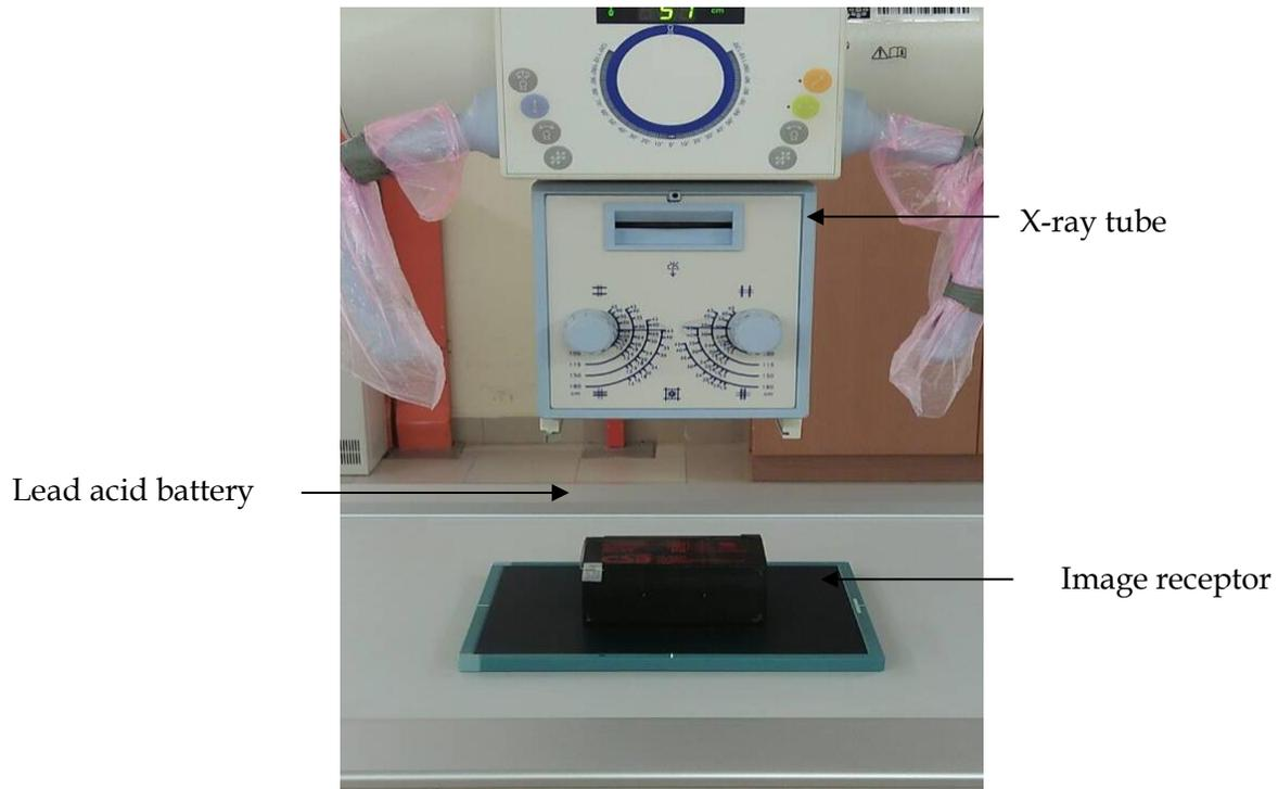
**Figure 1.** The arrangements of the image receptor and lead acid battery to the x-ray tube during exposure to the radiation
