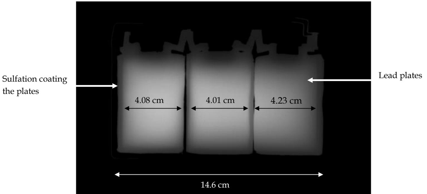
**Figure 3.** Front view of lead acid batter exposed at 125 kVp and 15 mAs
