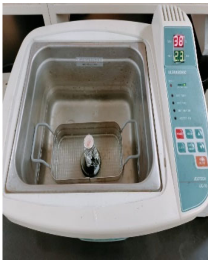
Figure 2: Preparation of 100% US extract by ultrasound-assisted extraction method.
