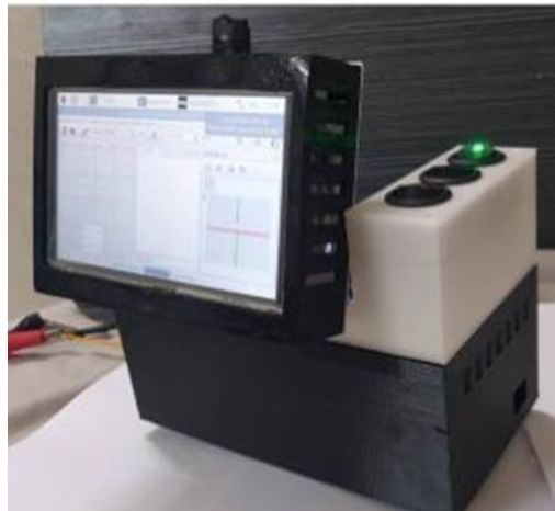
Fig. 3. Raspberry PI based onboard controller for the CNC system
