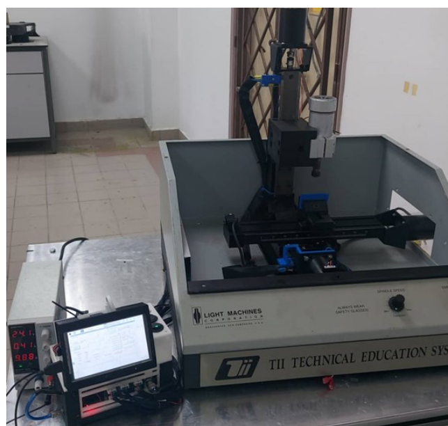
Fig. 4. Modular controller hosting the GUI to operate the CNC machine
