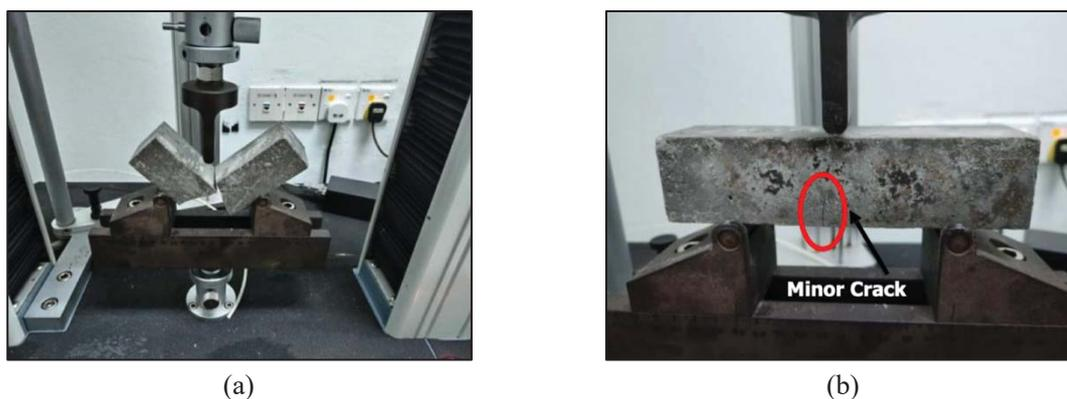
Fig. 11: The conditions of the (a) control and (b) AC-CF specimens after failure.
