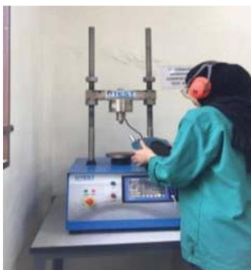
Fig. 2: Marshall testing.
