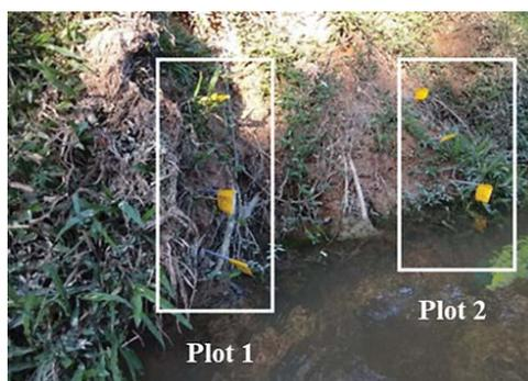
Fig. 3: Erosion pins installed at the site.
