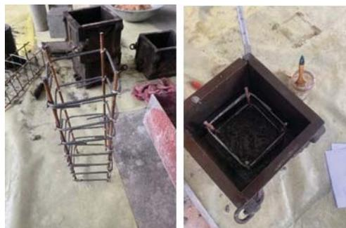
Fig. 3: Steel reinforcement of RC columns.
