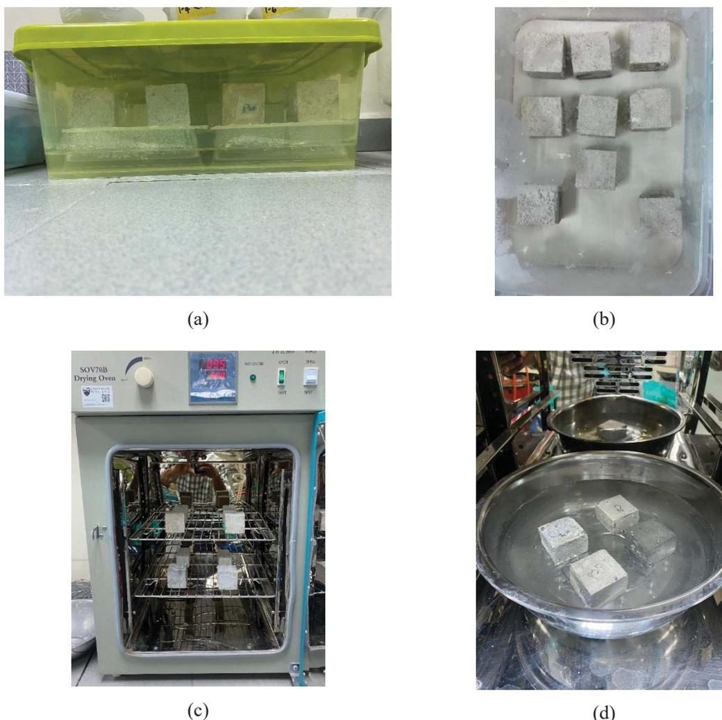
Fig. 3: Curing conditions in (a) saturated conditions, (b) saturated lime water, (c) hot air and (d) hot water.
