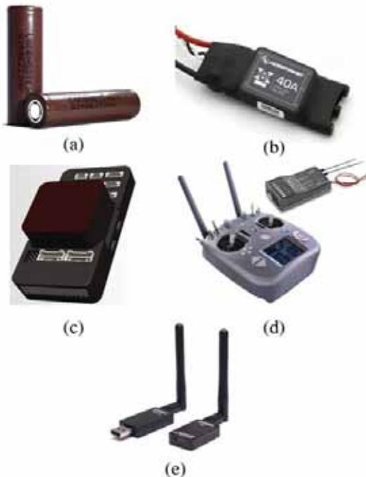
Fig. 5: (a) Li-ion battery (b) ESC XRotor-40A (c) Pixhawk 2 CAD model (d) TTSRC X9 (e) 3DR radio telemetry
