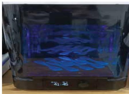
Fig. 3: Tensile test specimens during the post-curing process in Formlabs UV chamber (Formcure).
