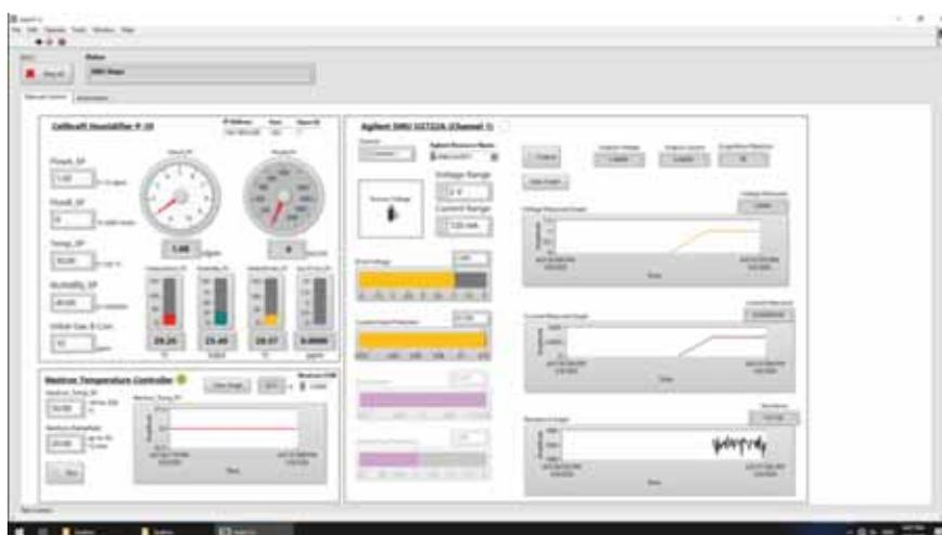
Fig. 2. Manual control of LabVIEW Gas System.
