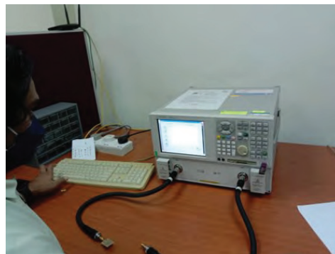
Fig. 15: Measurement of miniaturized antenna using Vector Network Analyzer.
