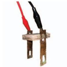
Fig. 4: The developed conductivity sensor.
