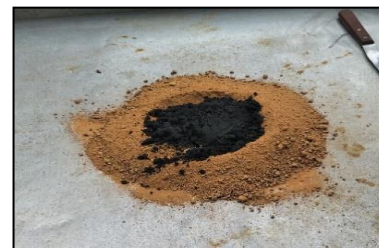
Fig 7: Preparation of geopolymer mixed with laterite soil.
