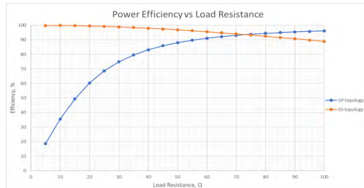
Fig. 9: SS and SP simulation for power efficiency, \eta vs load resistance, \Omega .
