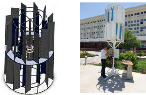
Fig. 3: External view of the wind power plant.
