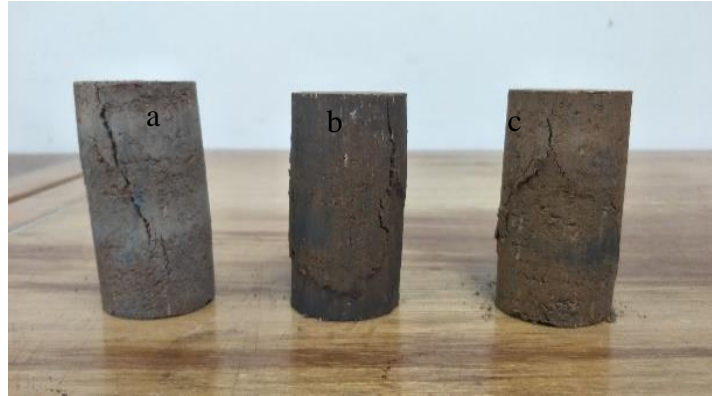
Fig. 11: (a) zero days, (b) seven days, (c) twenty-eight days of UCT.
