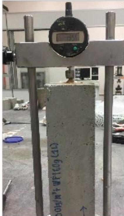
Fig. 4: Setup for drying shrinkage test.
