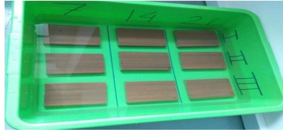
Fig. 2. Cellulose fibre reinforced HDPE layered silicate nanocomposites immersed in water for ageing.
