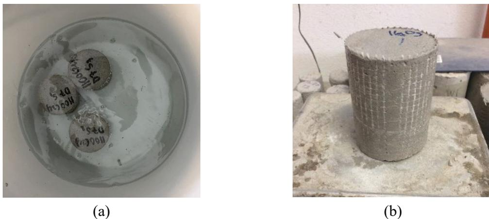
Fig. 2 :Water absorption test. (a) LFC specimens were fully submerged in a water tank, (b) Side view of LFC specimen.
