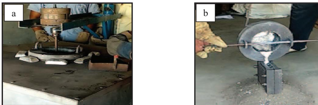
Fig. 3: (a) Stirring of molten metal and (b) Pouring the molten metal in to the die.
