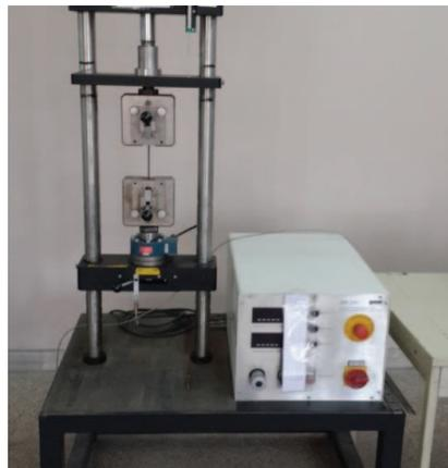
Fig. 7: Compressive strength test machine.
