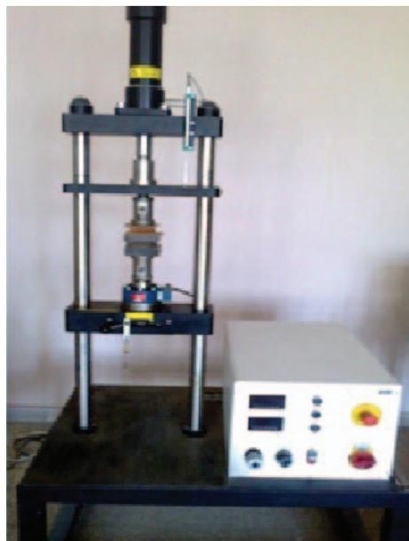
Fig. 8: Sample under compressive strength test.
