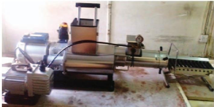
Fig. 4: Clay extrusion device.
