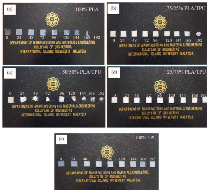
Fig. 6. Physical change of specimens after predetermined time of immersion in alkaline solution for (a) neat PLA, (b) PLA/TPU 75/25, (c) PLA/TPU 50/50, (d) PLA/TPU 25/75, and (e) neat TPU.
