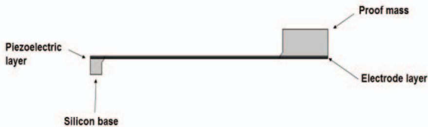
Fig. 1: Cross section of MEMS piezoelectric energy scavenger with proof mass.
