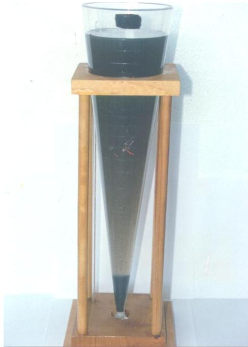
Fig. 7: Sludge Volume Index (SVI) Test.
