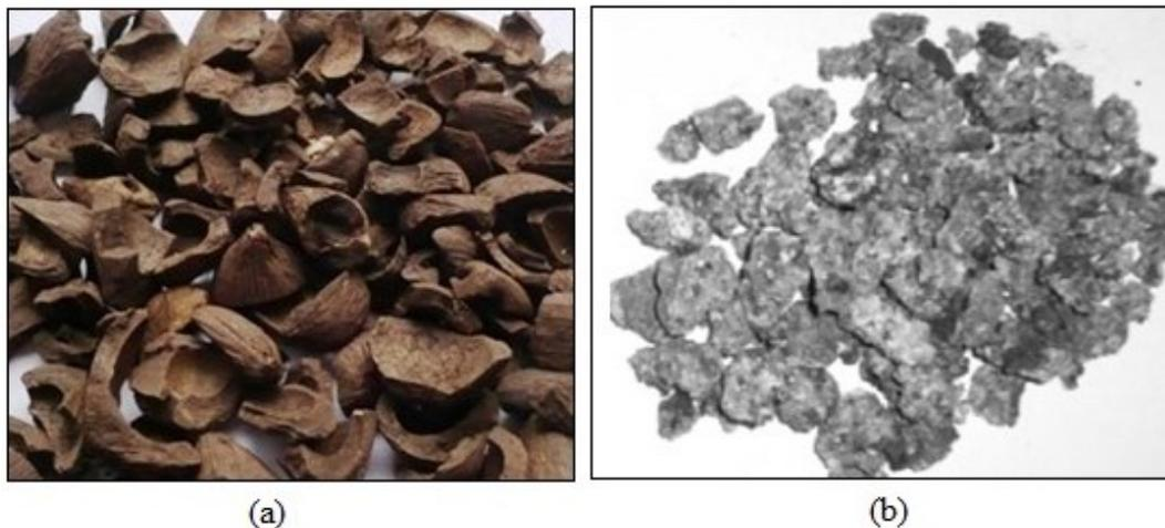
Fig. 1: Local waste (a) OPS as coarse aggregate; (b) POC as coarse aggregate.
