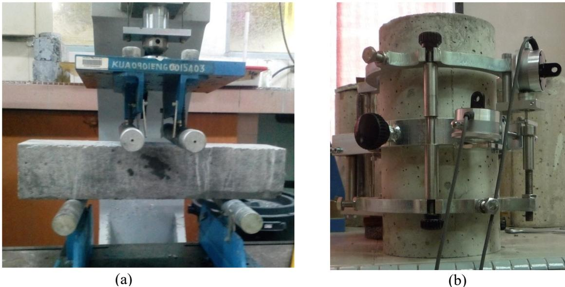
Fig. 2: Equipment setup for (a) the flexural strength test, (b) the compressometer for  $E_s$ .
