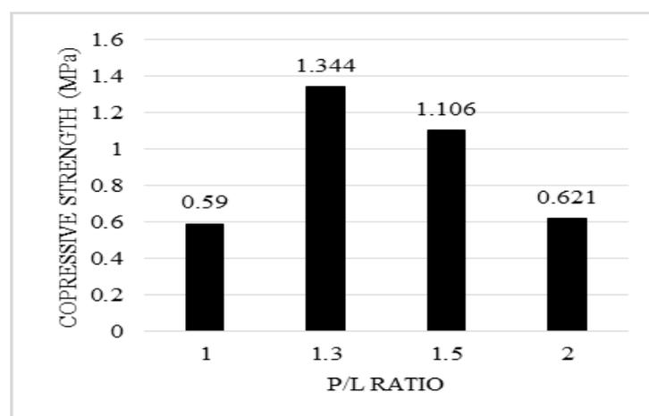
Fig. 9: Compressive strength of CPC with various P/L ratios.
