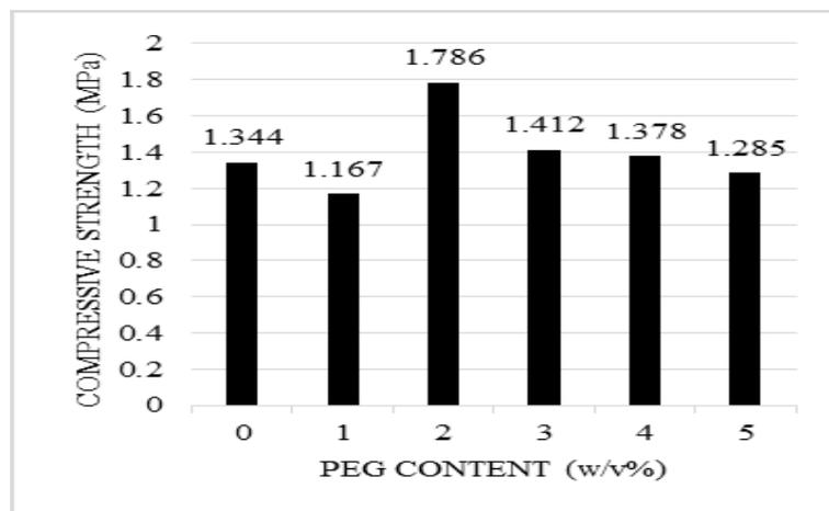
Fig. 10: Effect of PEG addition on the compressive strength of CPC prepared with the P/L ratio of 1.3.
