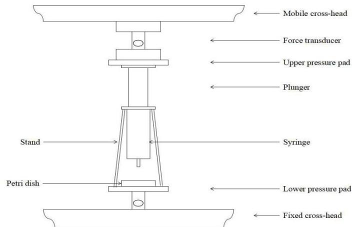
Fig. 1: Schematic diagram of the injectability test.
