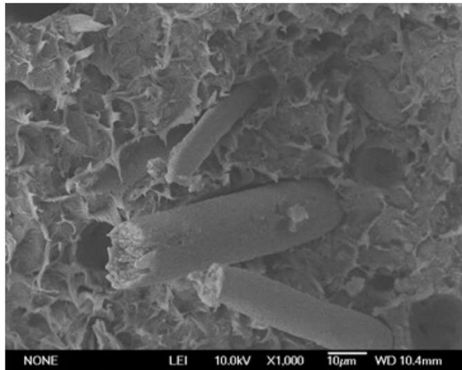
Fig. 6: FESEM micrograph of PP/DSNF composite after UV radiation.
