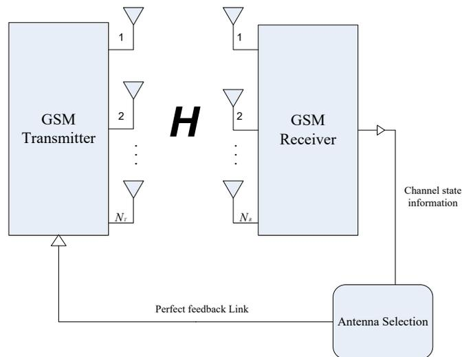
Fig. 2: System model for the proposed LC-GSM system.
