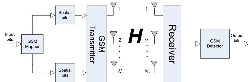
Fig. 1: System model for a conventional GSM system [4].
