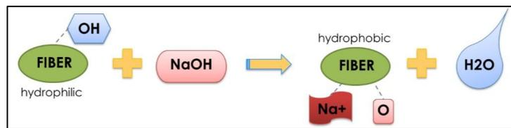
Fig. 7: Mechanism of alkaline treatment process.
