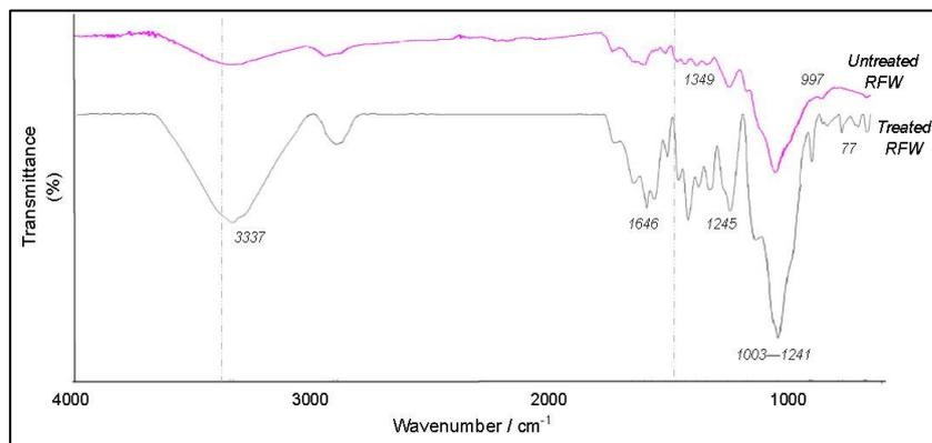
Fig. 2: Comparison of FTIR spectra of untreated and treated RFW.
