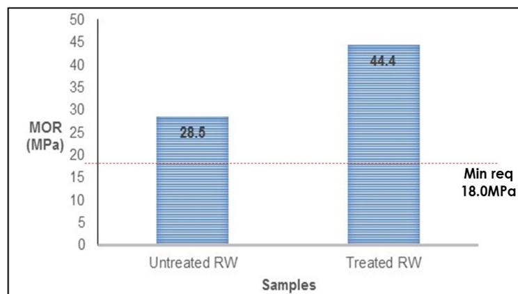
Fig. 4: Graph of Modulus of Rupture (MOR) for untreated and treated BPB panels.
