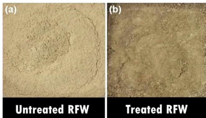
Fig. 1: Pictures of (a) untreated and (b) treated RFW fibres.
