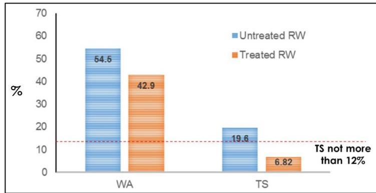
Fig. 6: Graph of dimensional stability of untreated and treated BPB samples.
