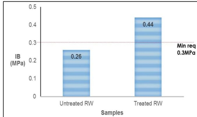
Fig. 5: Graph of Internal Bonding (IB) for untreated and treated RFW BPB.
