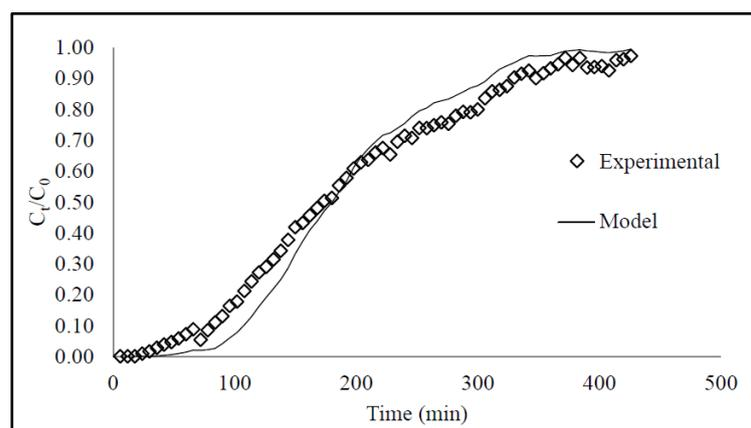
Fig. 3: Mathematical modelling using Belter equation. The experiments were done with a bed height ( $Z$ ) of 10 cm, volumetric flow rate ( $Q$ ) of 5 mL/min, and initial vanillin concentration ( $C_0$ ) of 900 mg/L.
