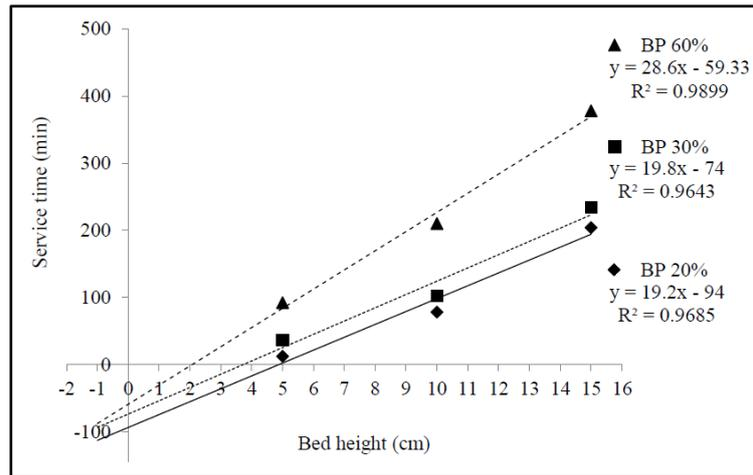
Fig. 2: Bohart-Adams model for different breakthrough points (BP) at different bed heights, constant flow rate (5 mL/min), and constant vanillin initial concentration (1,000 mg/L).
