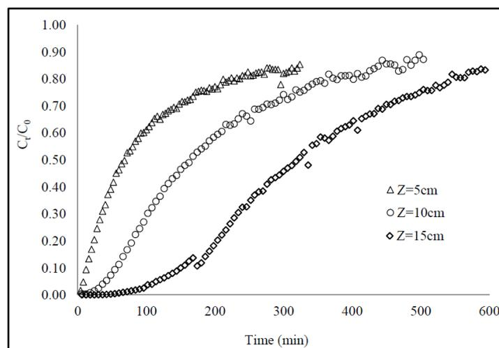
Fig. 1: The effect of bed height on breakthrough curves for vanillin adsorption onto resin H103.
