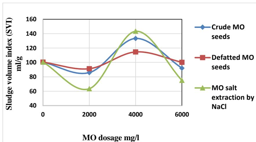
Fig. 2: Different MO coagulant-forms and their SVI values at different dosages.
