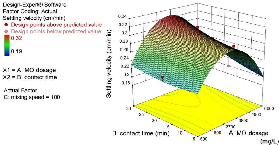
Fig. 4: The 3D contour plot of the interaction of dosage with contact time at mixing speed of 100 rpm.
