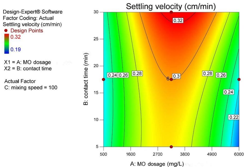
Fig. 3: The 2D contour plot of the interaction of dosage with contact time at mixing speed of 100 rpm.
