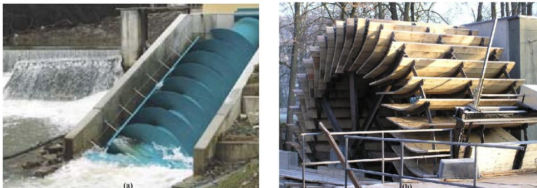
Fig. 1: Two ways of generating electrical energy from water: (a) hydrodynamic screw system, (b) water wheel system [1].
