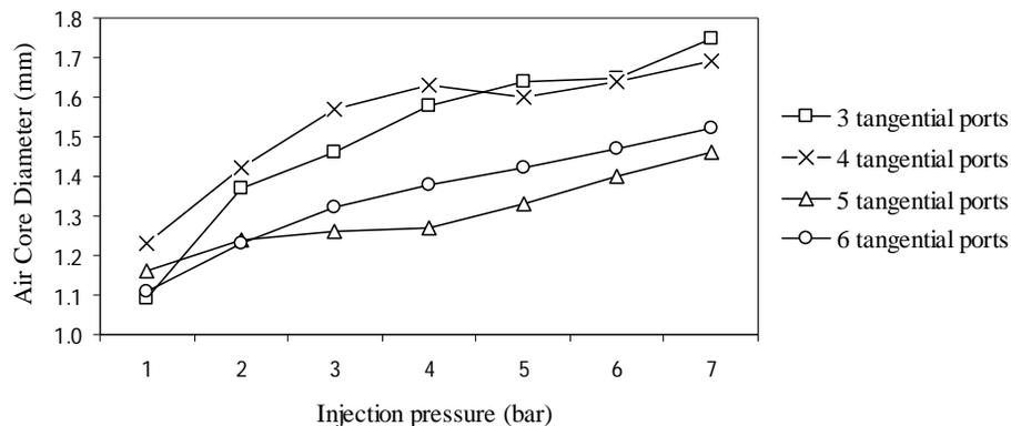
Fig. 7: Effects of injection pressure and number of tangential ports on air core diameter.
