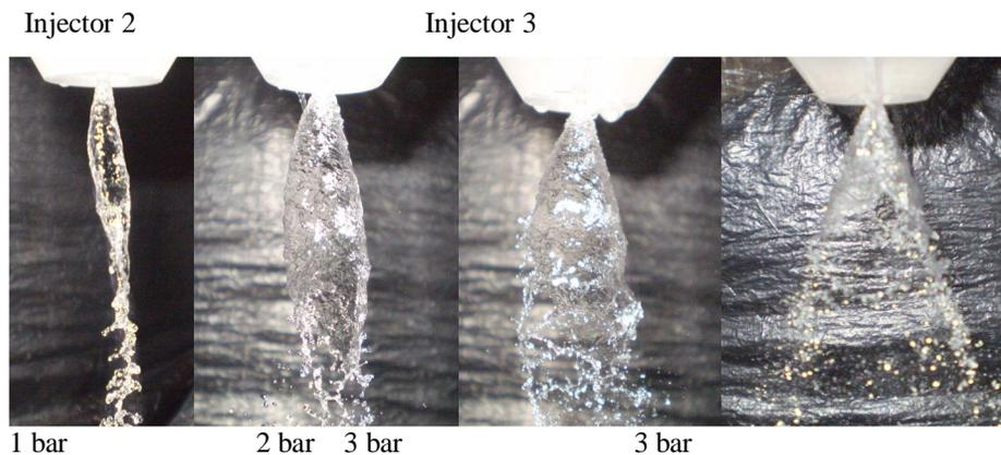
Fig. 6: Different stages of sprays.
