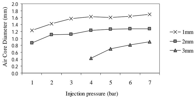
Fig. 9: Effects of injection pressure and diameter of tangential ports on air core diameter.
