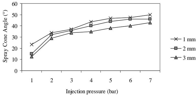
Fig. 8: Effects of injection pressure and diameter of tangential ports on spray cone angle.
