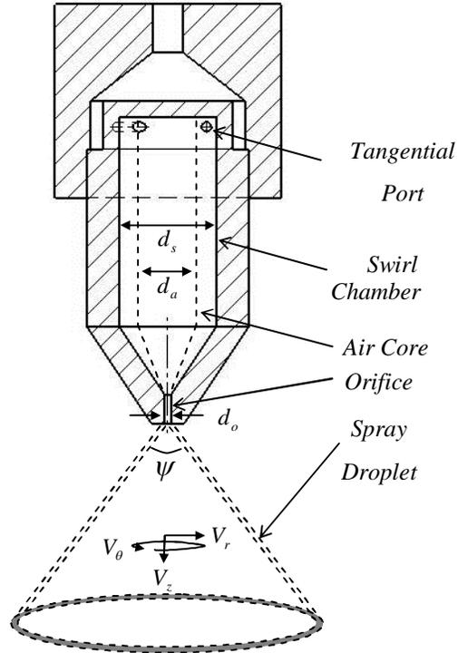
Fig. 1: Schematic sectioning of hollow cone swirl injector.
