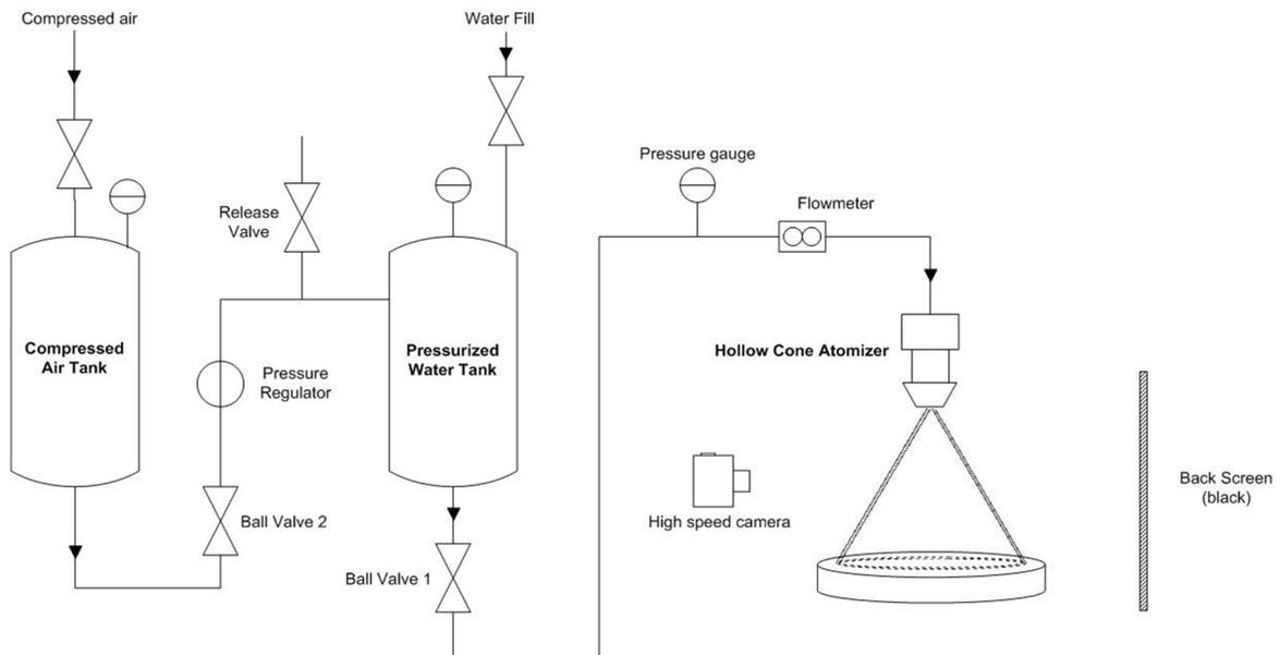
Fig. 2: Line diagram of the experimental setup.
