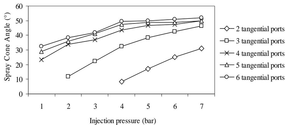
Fig. 5: Effects of injection pressure and number of tangential ports on spray cone angle.
