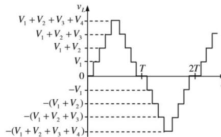
Fig. 1: N-levels waveform on multilevel inverter output (9-levels).
