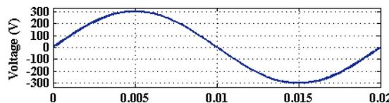
Fig. 9: The waveform of output voltage for the second cascade topology (169 levels) (simulation).
