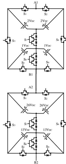
Fig. 5: The second proposed cascade topology (two unit).
