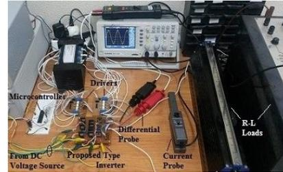
Fig. 11: Picture of experimental setup in laboratory.
