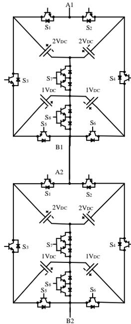
Fig. 4: The first proposed cascade topology (two unit).
