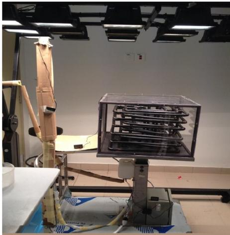
Fig. 3: Experiment setup with solar simulator at angle of 90°.
