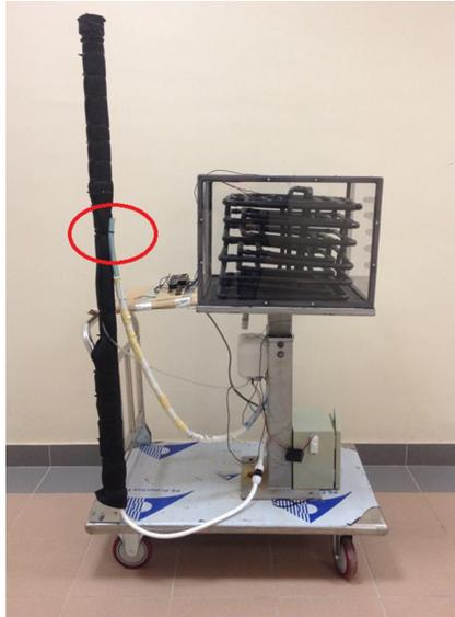
Fig. 5: Location of the clipped water channel.
