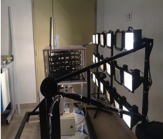
Fig. 1: Experiment setup with solar simulator at angle of 0°.
