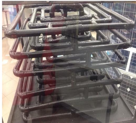
Fig. 4: Multilayered absorber in solar collector.
