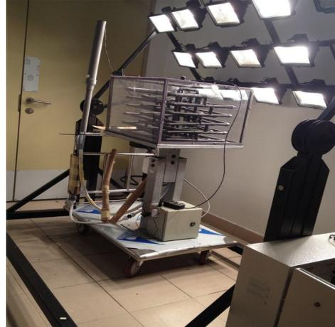
Fig. 2: Experiment setup with solar simulator at angle of 45°.
