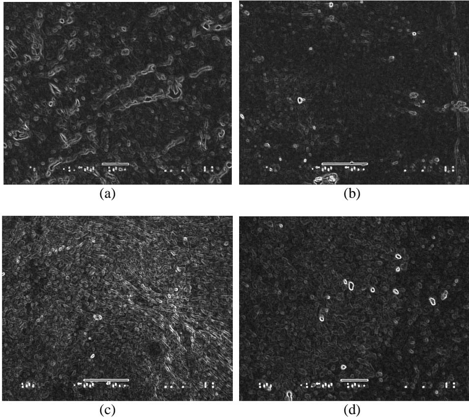
Fig. 5: SEM micrograph of (a) 5 wt% (b) 10 wt% (c) 15 wt% (d) 20 wt% of Copper oxide in ER-CuO solution.
