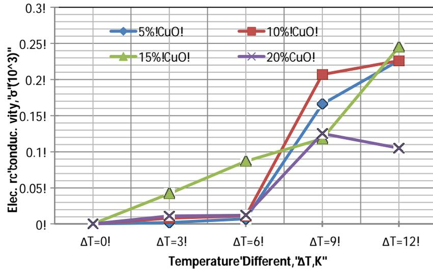
Fig. 6: Electric conductivity vs temperature difference.
