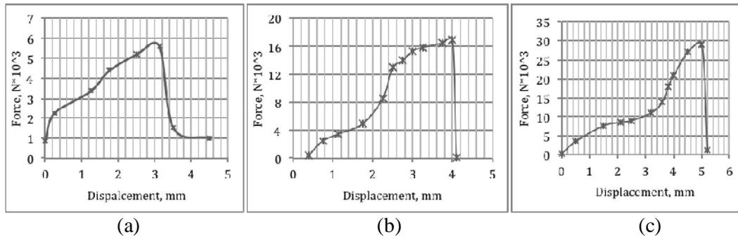
Fig. 2: Tensile test for force vs displacement, (a) Specimen #1 (woven plies 3), (b) Specimen #4 (woven plies 6), (c) Specimen #7 (woven plies 9).
