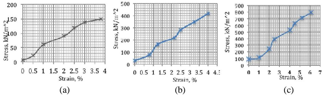
Fig. 3: Tensile test for stress vs strain, (a) Specimen #1 (woven plies 3), (b) Specimen #4 (woven plies 6), (c) Specimen #7 (woven plies 9).
