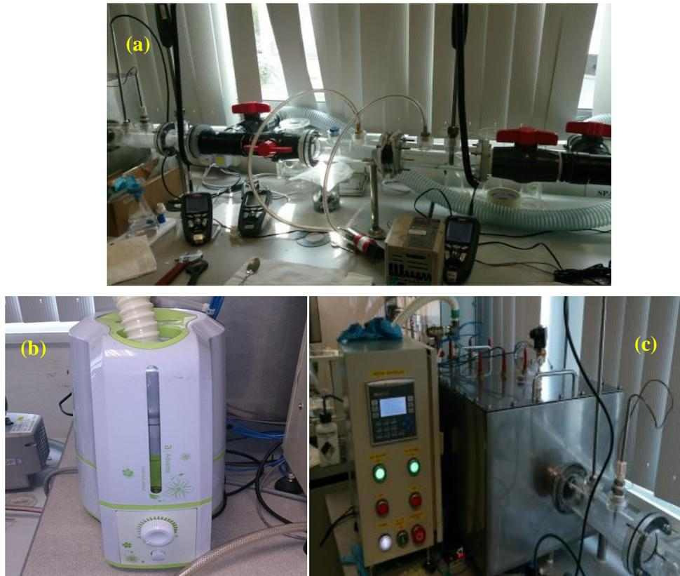
Fig. 2: (a) A pictorial view of the actual small-scale system setup; (b) a condition chamber with system controller; (c) a humidifier to regulate the humidity of the inlet air to the experimental setup.
