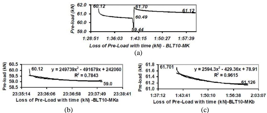
Fig. 6 Loss of Pre-load with Time for Bolt 10 with Molykot lubricant. (a) Overall tightening, (b) First tight, (c) First Re-tight.
