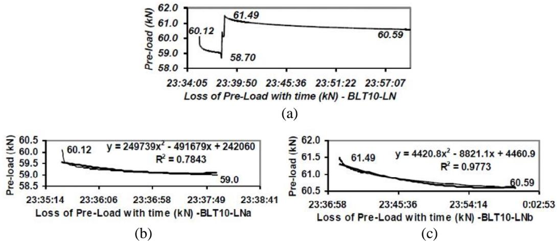
Fig. 7: Loss of Pre-load with Time for Bolt 10 with Locknut. (a) Overall tightening, (b) First tight, (c) First Re-tight.
