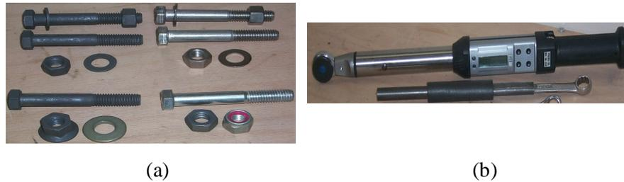
Fig. 2 (a) Bolts, nuts and washers used during tests, (b) Tools (torque wrenches) used.
