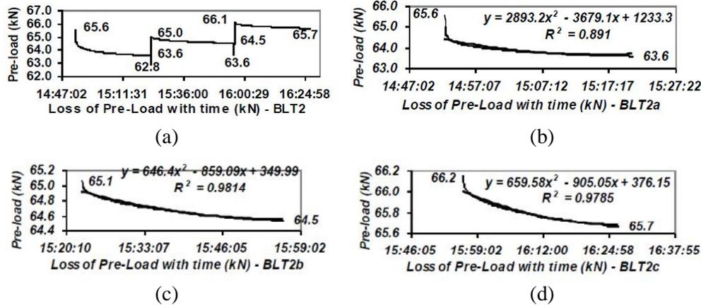
Fig. 3: Loss of Pre-load with Time for Bolt-2. (a) Overall tightening, (b) First tight, (c) First Re-tight, (d) Second Re-tight.
