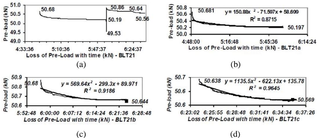
Fig. 8 Loss of Pre-load with Time for Bolt 21. (a) Overall tightening, (b) First tight, (c) First Re-tight, (d) Second Re-tight.
